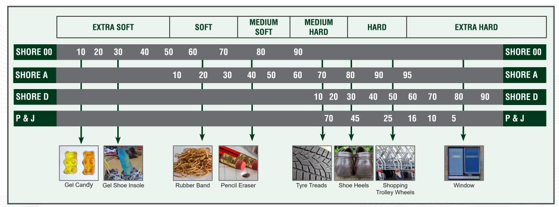
**Erapol** elastomers are available in a wide range of hardness, from 10 Shore A, which is softer than an eraser, to 85 Shore D which is much harder than a golf ball.
